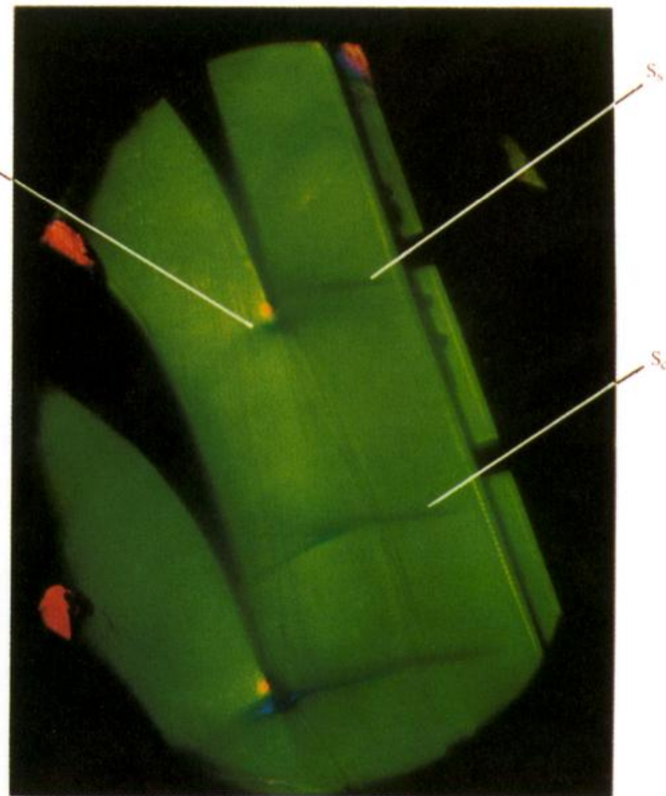
Figure 12. Test L3: dry inflow, \Delta T_0 = 7.5^\circ\text{C} , M_{2s} = 1.08 , porous tailboard.
